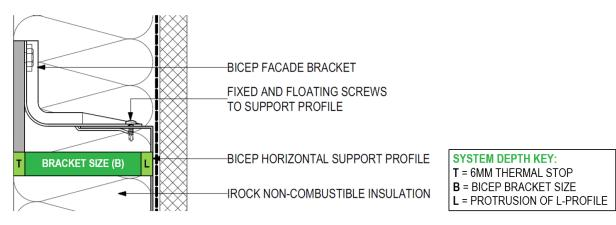
**Important Note:** To achieve a thermally broken system as per section **4.1** above, it is necessary to use all the above brackets in combination with the *BCTBS6 Thermal Break Spacer* which is 6mm thick. In this case, add 6mm to all the above depth measurements.
