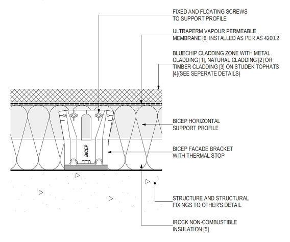
**Important Note:** The location of the ULTRAPERM membrane on the outside of the insulation (as shown here) or the inside between the bracket and the structure will depend on the project climate zone, the wall-build up, the cladding system and other project specific considerations.
